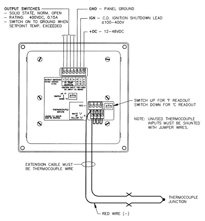
NOTE: ALL EXTENSION WIRE CONNECTIONS MUST BE OF THE SAME METAL. ALL CONNECTIONS TO BE CLEANED, TIGHTLY TWISTED AND INSULATED WITH CERAMIC WIRE NUT.
