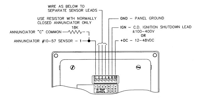
NOTE: FOR INTRINSICALLY SAFE OPERATION, POWER FROM ALTRONIC 690 107/108 BARRIER FOR IGNITION POWER OR FROM A CSA CERTIFIED ZENER BARRIER RATED 30V MAX., 120Ω MIN. FOR DC POWER.
