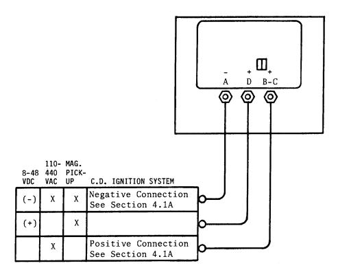
NOTE: Only one (1) positive connection used to either D or B-C terminal as shown.
