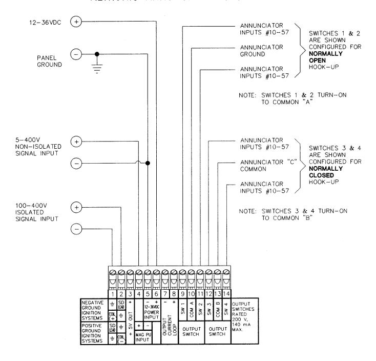
NOTE: FOR INTRINSICALLY SAFE OPERATION, POWER THROUGH A CSA CERTIFIED ZENER BARRIER RATED 30 VOLTS MAX., 1200 MIN. THE SIGNAL INPUT, IF FROM THE IGNITION COIL OR THE SHUTDOWN LEAD, MUST BE RUN THROUGH AN ALTRONIC BARRIER 690 107 OR 690 108. FOLLOW THE INSTALLATION INSTRUCTIONS SUPPLIED WITH THE BARRIERS.
