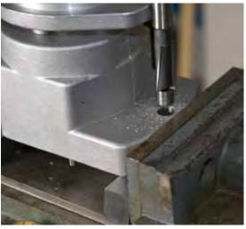
**STEP 2:** Using a 9/16" counter-bore with a 7/16" pilot, spot-face the O-ring sealing surface. Remove just enough material to provide a smooth surface.
